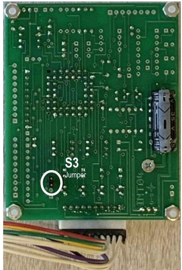
Address Jumper S3 on back of front cover
