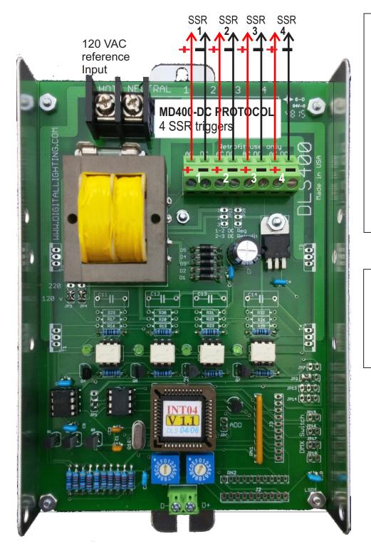
The MD400-DC SOLID STATE RELAY trigger control is compatible with **PROTOCOL** Digital lighting control systems
