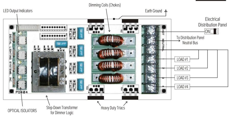
For Full Load Operation Use: #12 AWG copper conductor wire for Line & Neutral Feeds. #14 AWG copper conductors in/out to each load. Max. Load: 4 Amperes (480W at 120 VAC, 880W at 220VAC) per output.
