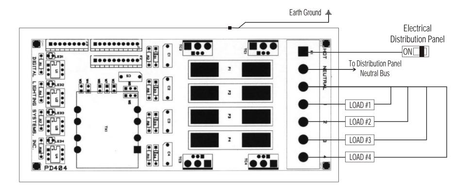
For Full Load Operation Use: #12 AWG copper conductor wire for Line & Neutral Feeds. #14 AWG copper conductors in/out to each load. Max. Load: 4 Amperes (480W at 120 VAC).
